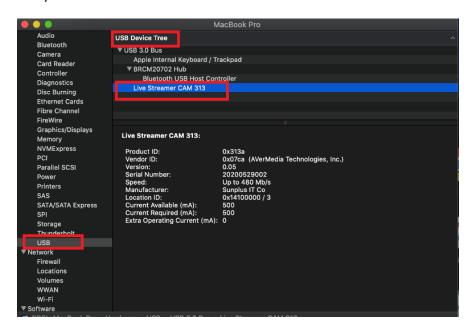
If it is listed in the USB devices, the Live Streamer CAM313 is successfully detected by your Apple computer.
