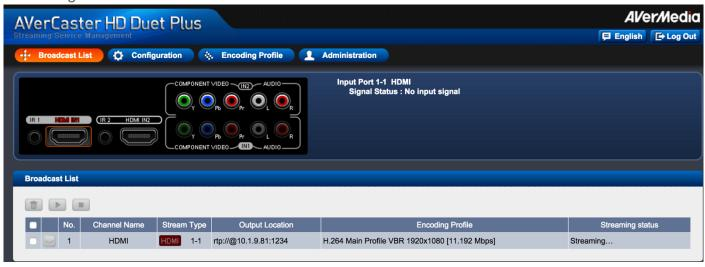
On computer 10.1.9.81, use VLC's "Open Network" and enter the URL to receive streaming.
