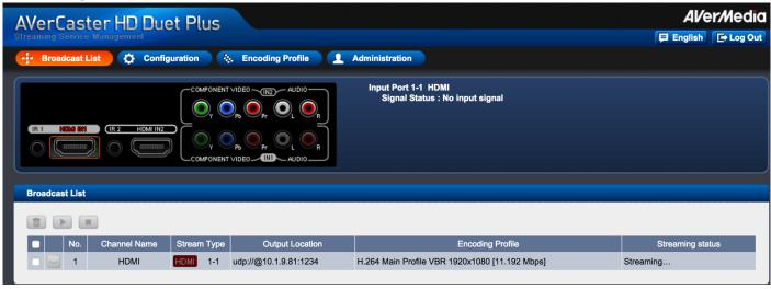
On computer 10.1.9.81, use VLC's "Open Network" and enter the URL to receive streaming.
