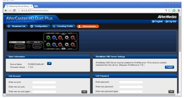
Below the four tabs are the input selection icons, which resembles the connectors in the back of F239+. They give you an intuitive way of selecting video and audio inputs by clicking on the connectors.
