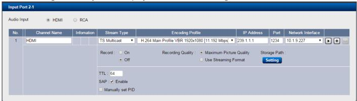
To receive this TS multicast streaming, go to "Broadcast List" and look up the "Output Location" for the streaming URL.
