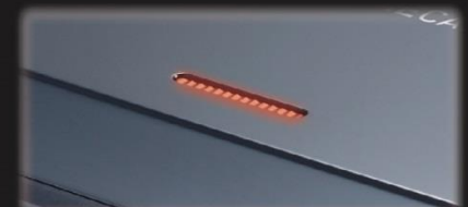
The LED indicator for recording/status
